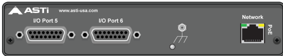
Figure 3: Rear panel of AI-Tango
