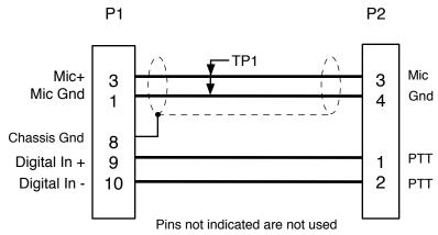
\*Application note: This cable is the -C variant for use with Electrovoice 903E hand-mics ONLY. Please confirm applicability for use with other hand-mics with ASTi engineering before use.
