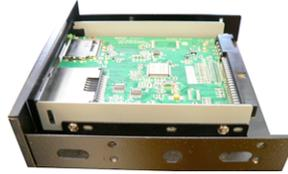
2. Insert screws on either side of the compact flash drive.
