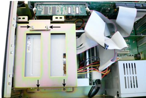
2. Remove the ribbon (IDE) cables by pulling them out of the back of the floppy drive and removable hard drive. Be sure to handle it carefully by grabbing the black plastic part securely and pulling.
