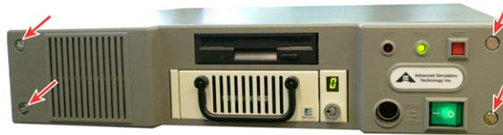
4. After loosening the screws, snap the front cover off the DACS.
