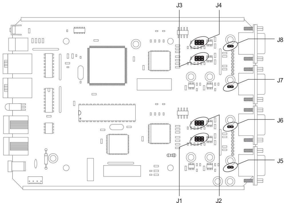
**Warning:** Take ESD precautions when handling the RIU board, EEPROM, or jumpers. When changing jumpers, first touch chassis ground, and then reposition the jumper.
