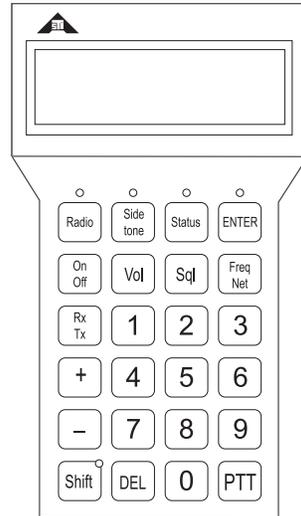
*Figure 12: Operator Station HHT Device*
