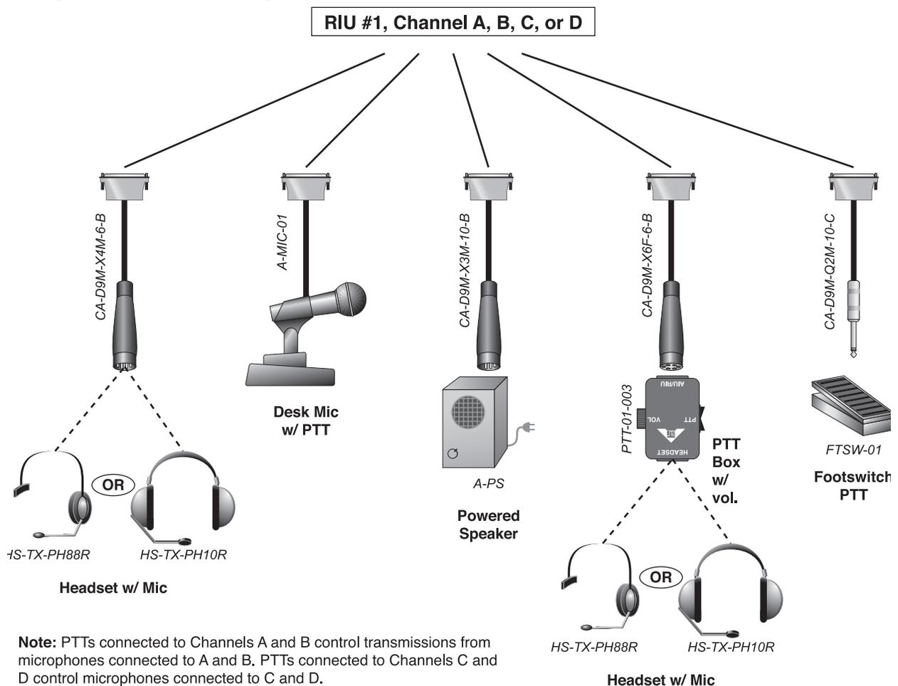
Figure 4: Operator Station Audio and Control Device Installation
