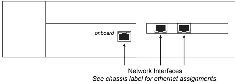
*Figure 2: 2U Telestra Chassis Ethernet Port Physical Locations*
