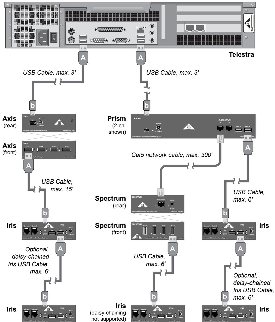
Figure 5: Master USB Connection Diagram
