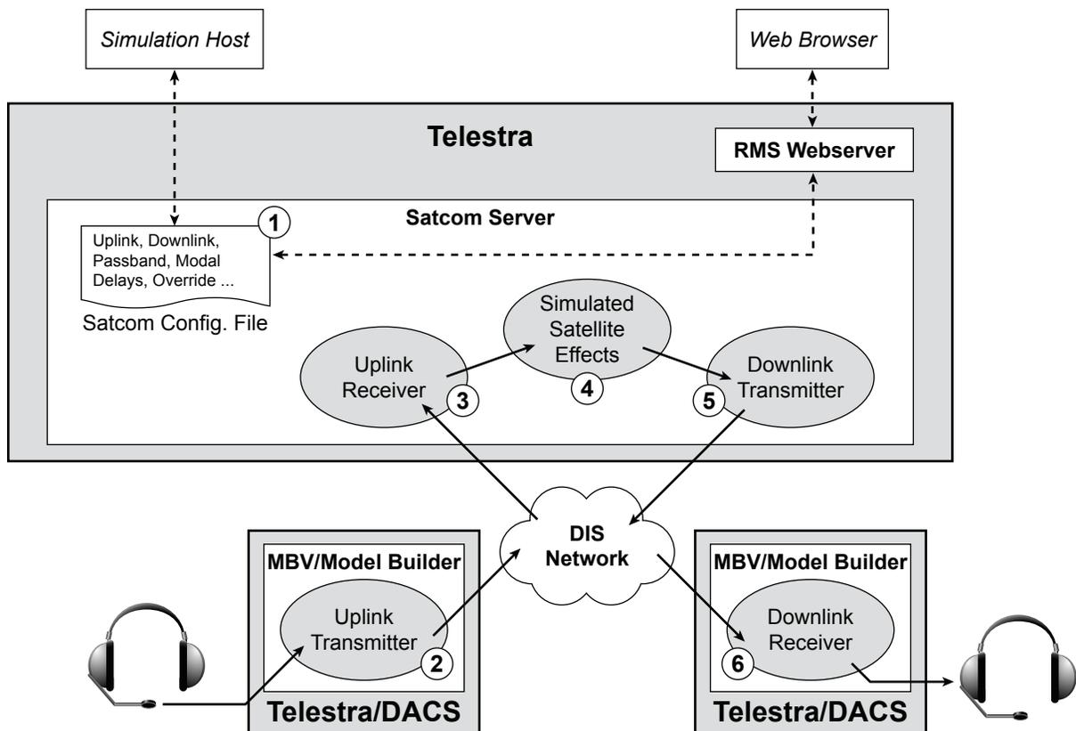
Figure 100: ASTi Simulated Satellite Communications System Functional Flow Diagram
