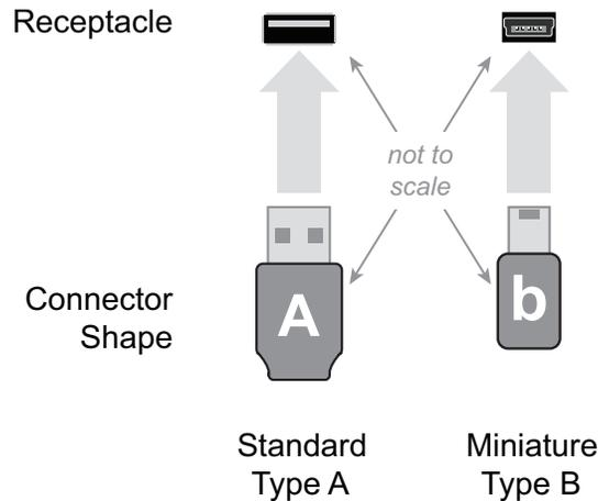
*Figure 3: USB Cable Connector Identification*
