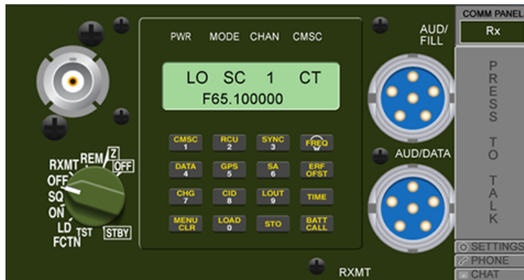
Figure 284: PRC-119 ASIP faceplate
